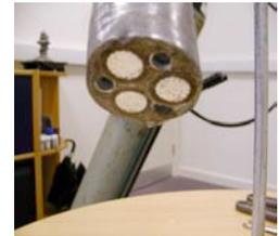
AES Hydrogel Purging System is a new and unique technology for the in-situ cleaning and purging redundant oil-filled power cables, oil feeder tanks and pipelines. They can then be safely left underground or removed at a later date without further contamination to the environment. The recovered oil is uncontaminated by our process and can be safely re-cycled.
